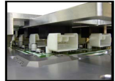
Close Up Showing Connector Alignment
